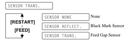
After selecting the sensor type, press the **[PAUSE]** key to go to Printing Mode Selection.
